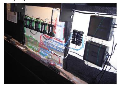
The picture on the left shows the situation at the rear wall (background) with the feedback sensors, to track occupancy report, the relay, the interface and the amplifier. In track or block diagram of the actual track Rocomotion course has been entered. There have been created 14 traffic boxes. All blocks are called traffic boxes. In the traffic boxes detectors can be created and trains are assigned. It can brake and / or stop indicators, and occupancy detectors will create.
